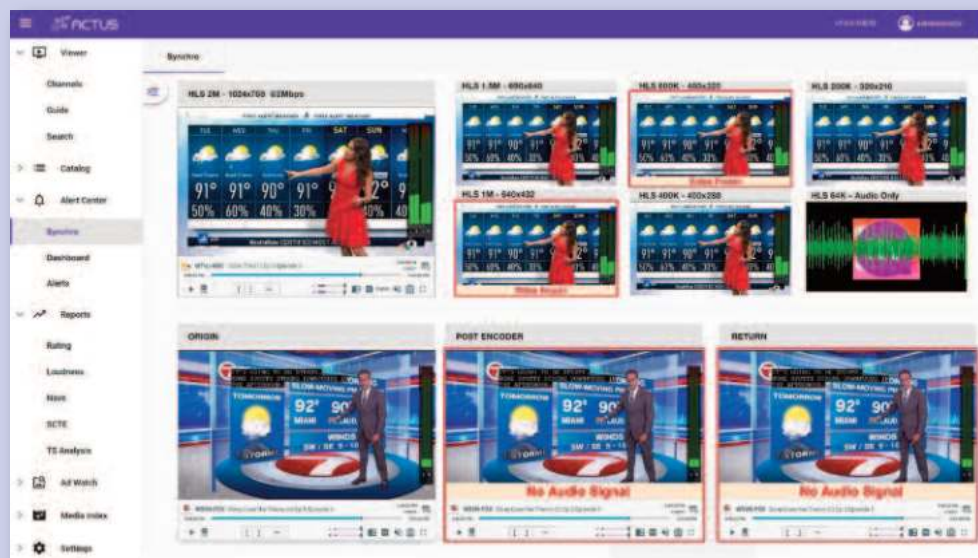
Actus Synchro pinpoints where errors are entering their video distribution chain and identify which renditions in an OTT ABR set are problematic.
